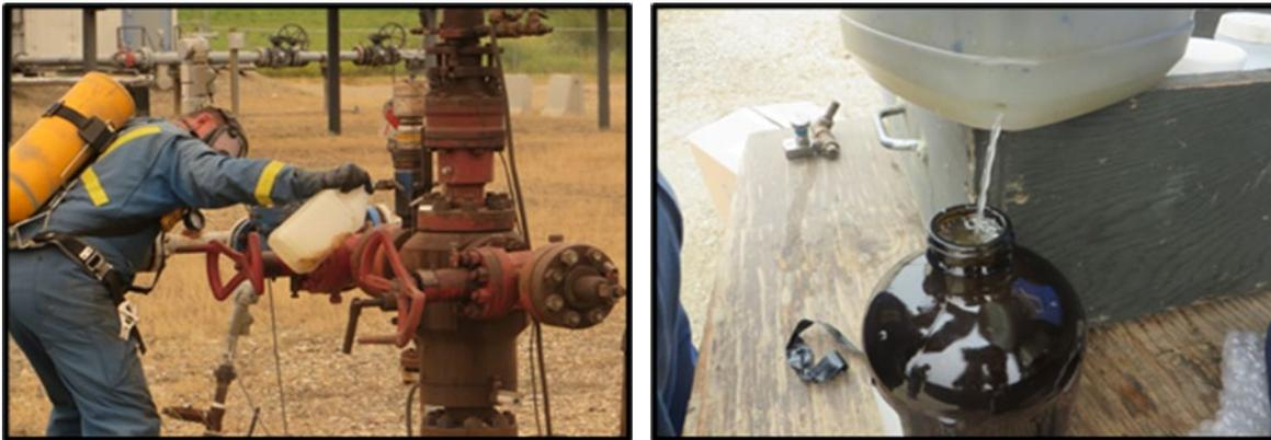
Figure 19: Sample Collection at Wellhead
