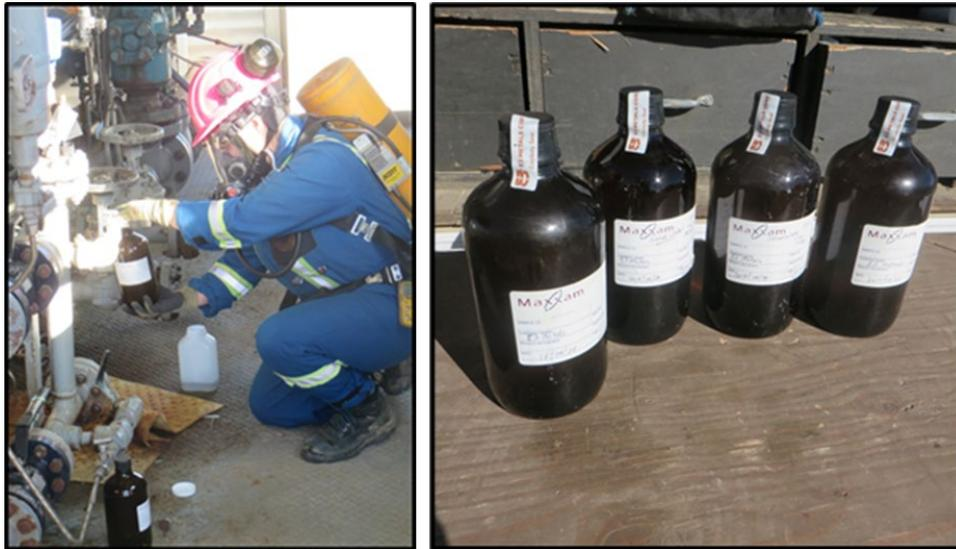
*Figure 21: Sample Collection at Test Separator*
